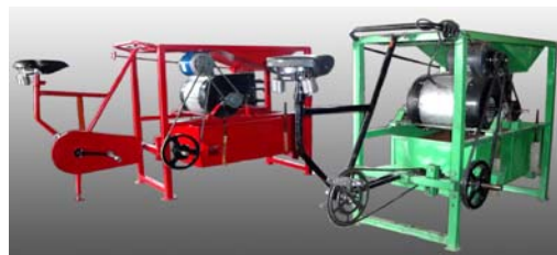
Commercial model of cleaner grader Developed by M/s Captain Tractors Pvt Ltd
